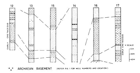
Text-fig. 2-Stratigraphic section through shallow wells.
