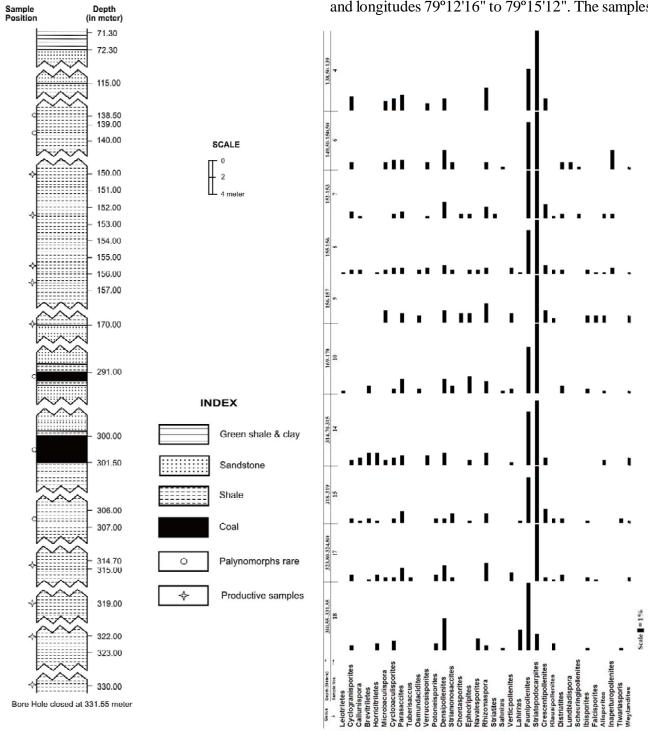
Fig. 3—Lithological details of the samples collected from Bore hole No. MR-157, Makardhokada area, Nagpur District, Maharashtra (Courtesy, DGM, Nagpur).
