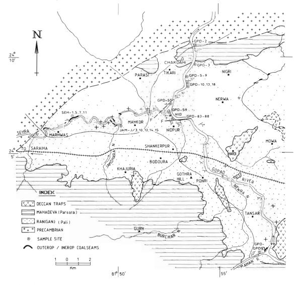
Map 2—Geological map of north-west portion of Singrauli Coalfield showing Marhwas area where the Nidpur beds (asterisk) are situated. The yielding samples, marked by dot within a circle, are indicated along the traverses taken. NID (asterisk) indicates the position of sample nos. NID-4, 5, 8, 10, whose details are given in Map 3 (after Raja Rao, 1983).
