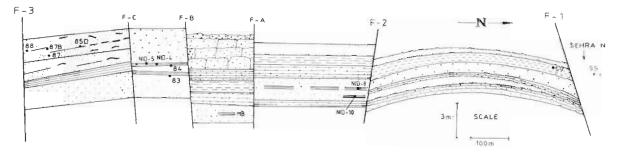
Text-figure 4- Generalised section of the Nidpur beds and associated sequence along Gopad River with location of palynologically productive samples (refer Map 3), F-1, F-2, F-3 major faults, F-A, F-B, F-C faults represented by minor dislocation (for Index sec Text-fig 5).
