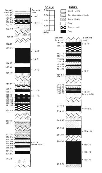
Text-figure 1—Showing position of coal samples studied from bore-hole no. 305.
