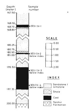
Text-figure 2—Showing position of coal samples studied from borehole no. 303.
