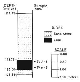
Text-figure 3—Showing position of coal samples studied from borehole no. 309.
