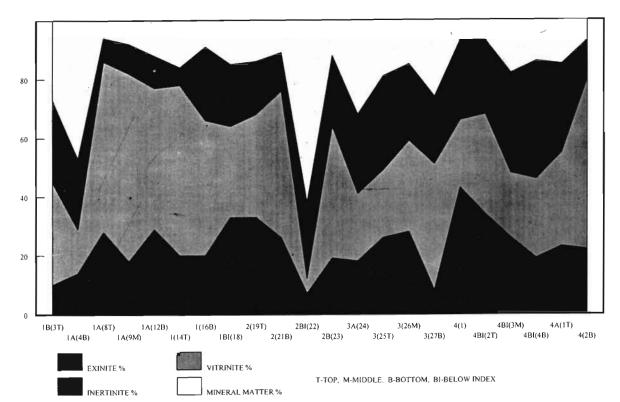
Text-figure 4-Maceral composition of coal seams in bore-hole nos. 305, 303 and 309.
