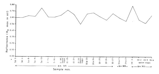
Text-figure 5-Showing reflectance analysis of coals from bore- hole nos. 305, 303 and 309.
