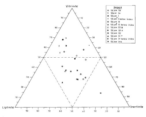
Text-figure 6—Showing triangular (m.m.f.) data plotting of coal macerals of bore-hole nos. 305, 303 and 309.
