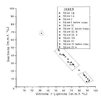
Text-figure 7—Showing biaxial (m.m.f.) data plotting of coal macerals of bore-hole nos. 305, 303 and 309.
