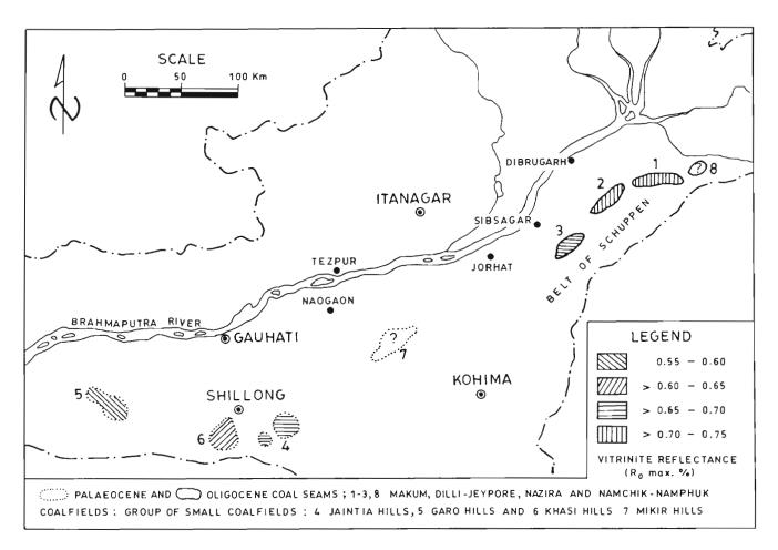
Fig. 8— Normal reflectance (R<sub>o</sub> max. %) trend in the Palaeocene and Oligocene coal seams of Arunachal Pradesh, Assam, Nagaland and Meghalaya (coalfield areas, especially of Meghalaya, are exaggerated for illustration) (after Misra, 1992a).
