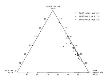
**fext-figure 5**—Ternary diagram showing composition of fluorescing and non-fluorescing macerals in the lignite seams of bore-holes NLE-27, 35 and 36.
