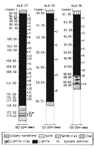
**Text-figure 3**—Core logs showing lignite seam and associated sediments along with position of samples in bore-holes NLE-27, 35 and 36.
