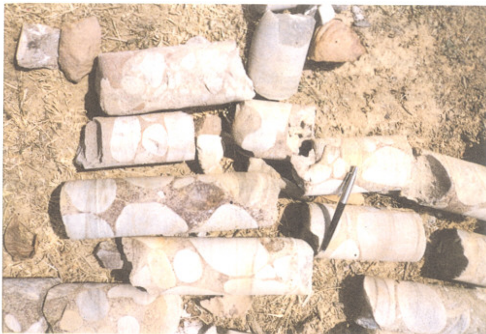
Bore-cores showing conglomeratic bed at the base of Barakar Formation, Talcher Coalfield, Orissa.
