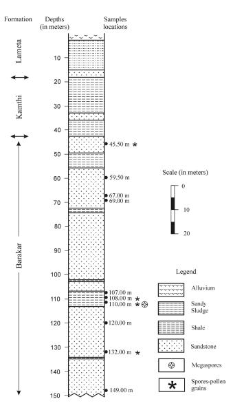
Fig. 2—Litho column of bore–core No. NP–75, Nand–Besur Block, Bandar Coalfield, Maharashtra showing position of samples.
