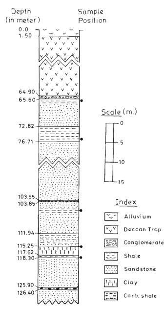
Fig. 2—Showing the levels of yielding samples in the lithological succession
